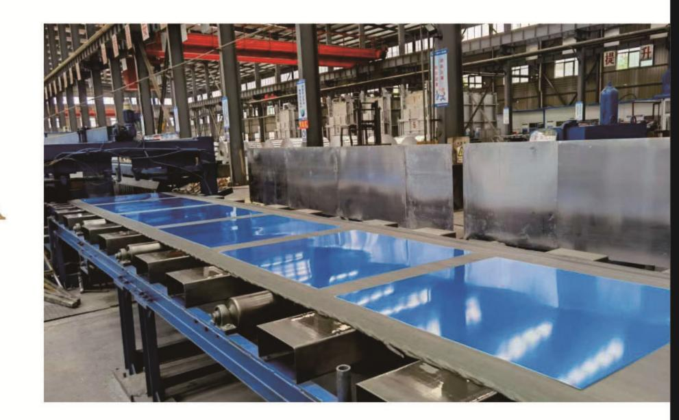
Our company has six flying shear units, all using advanced six-fold straightener equipment, so that the aluminum coil under the corresponding repeated bending to produce plastic deformation, remove the internal stress, elastic recovery, through unwinding, straightening and according to the set size of transverse shear, neatly stacked, high speed, high precision.
